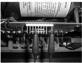
If the original Swell Shoe Simulator Switch is no longer available when you begin to set up your re-installed Peterson Model C Swell Shade Operator, you can simply use a clip lead to connect the Positive Common pin to each expression contact input pin, in turn, as shown in these photos.
